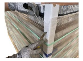
10. Remove the first corner piece by pulling down the piece.
