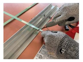
7. Cut the vertical straps (2. and 3.). Make sure you do not cut or damage the honeycomb or glass facing.
