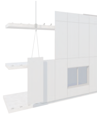
CLADITIZED SYSTEM Unitized Facade System
