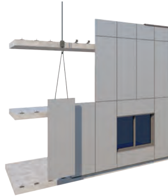
CLADITIZED SYSTEM Unitized Facade System
