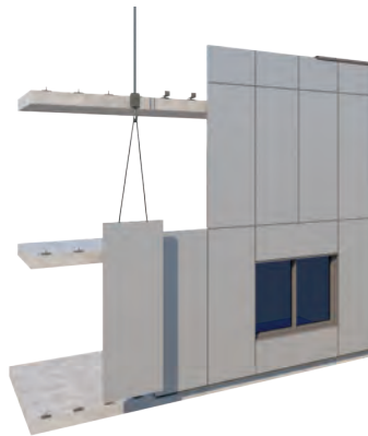
CLADITIZED SYSTEM Unitized Facade System
