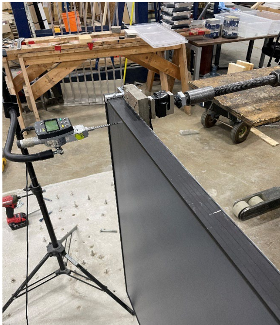
Adjacent to Post Horizontal Concentrated Load Test
