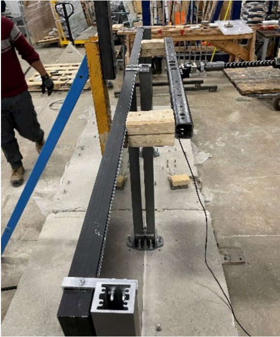
Horizontal Mid Span Concentrated Load Test (2-Bay)
