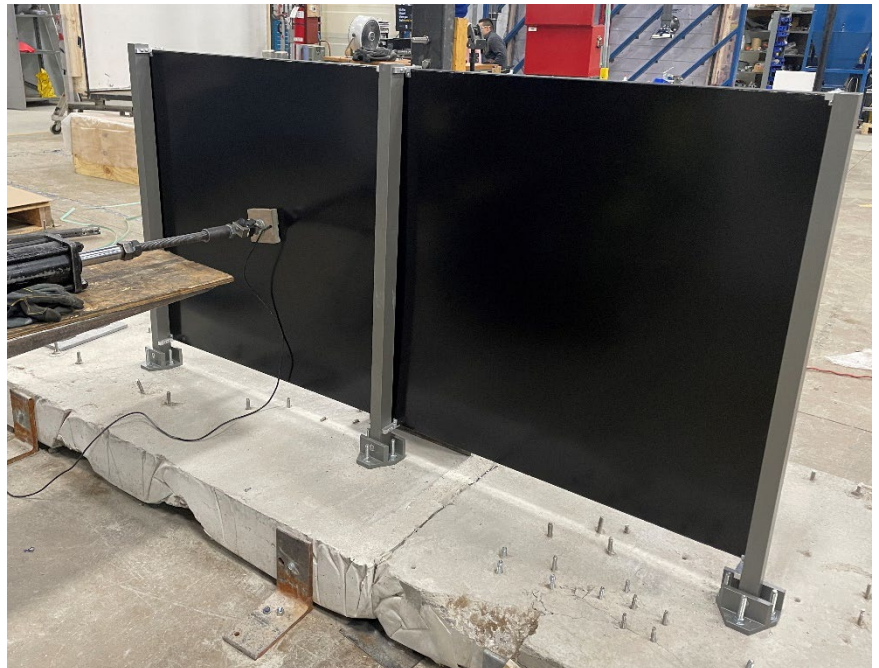
Infill Load Test
