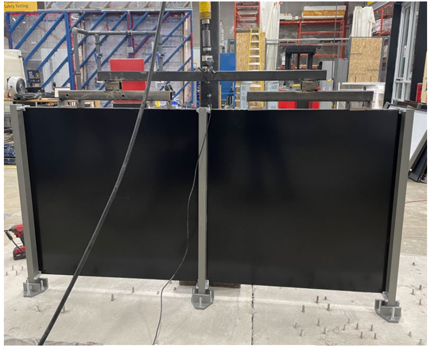
Vertical 1/4 Point/UDL Load Test
