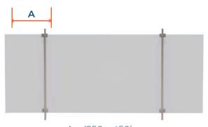
A = (250 – 450) mm Uplift Load ≤ 5400 Pa Downforce Load ≤ 5400 Pa
