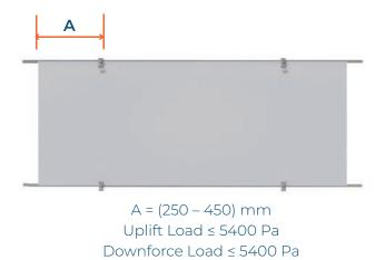
Clamp configuration CL2 – 4 point installation, mounting rails parallel to long edge of PV module.
