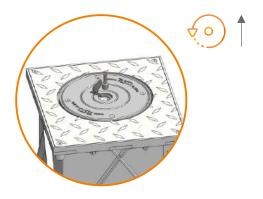
Turn the drill adapter contraclockwise to raised the bollard
