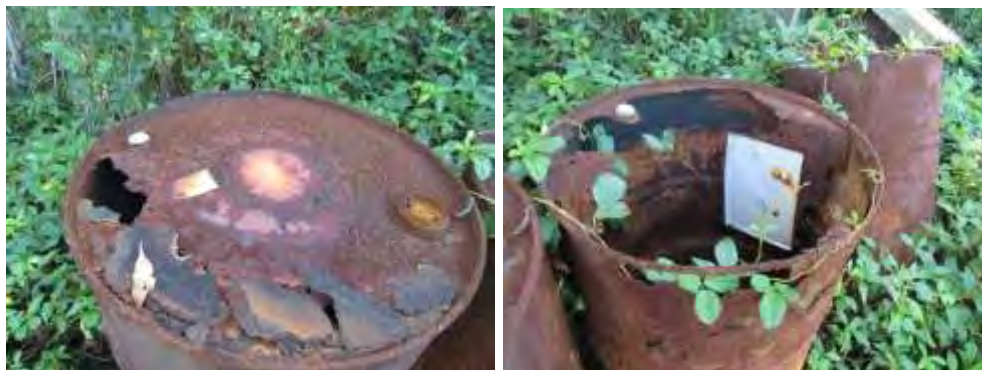
Photo 21: Corroded barrels with exposed material
