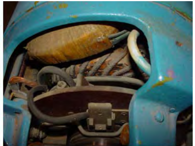
View of Compound Stator Coil and Slip Rings
