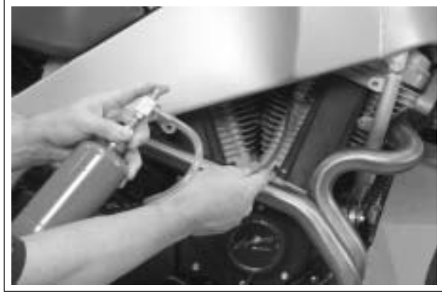
Figure 4-108. Checking for Intake Leak
