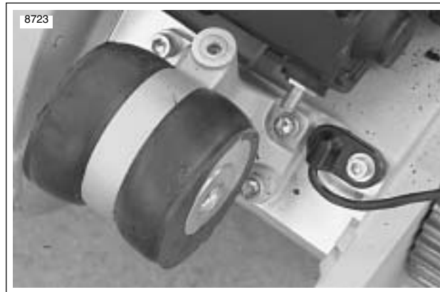
Figure 3-35. Rear Isolator and Mounting Hardware
