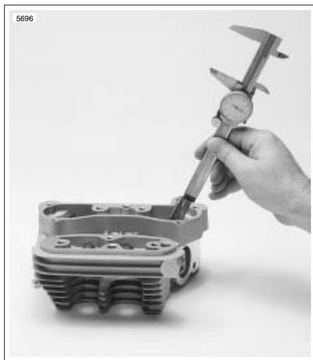
Figure 3-73. Measuring Valve Stem Protrusion
