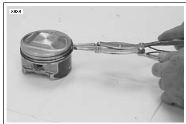
Figure 3-94. Removing Piston Rings
