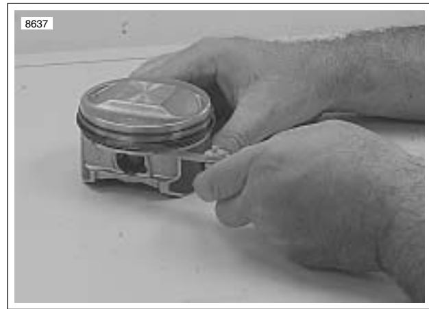
Figure 3-101. Measuring Ring Clearance in Groove
