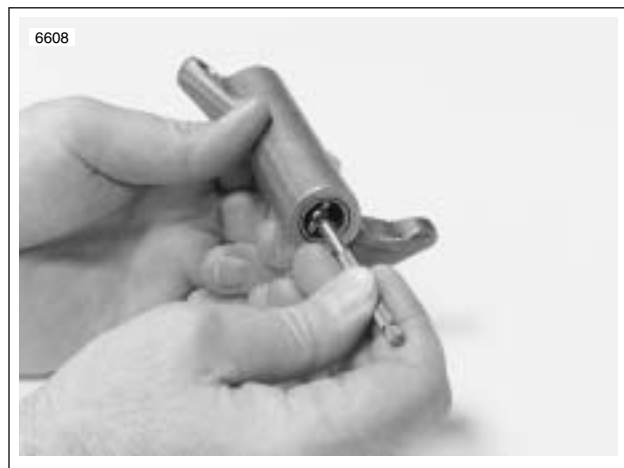
Figure 3-72. Measuring Rocker Arm Bushing Inner Diameter
