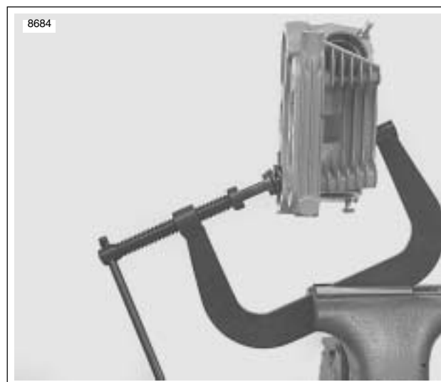
Figure 3-66. Valve Spring Compressor (Part No. HD-34736B)
