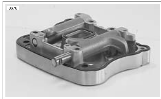
Figure 3-64. Removing Rocker Arm Shafts
