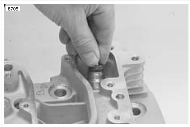
Figure 3-83. Valve Seal and Lower Collar Assembly Installation
