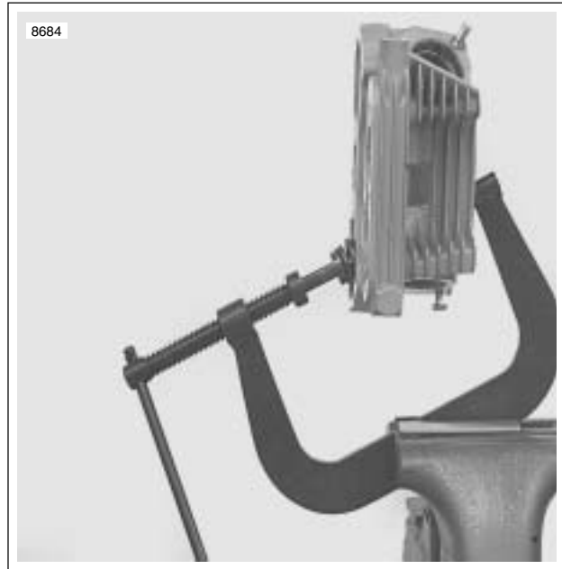
Figure 3-84. Valve Spring Compressor (Part No. HD-34736B)
