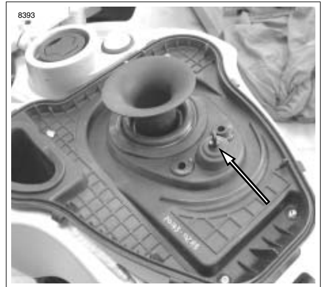
Figure 4-79. Intake Air Temperature Sensor Installed
