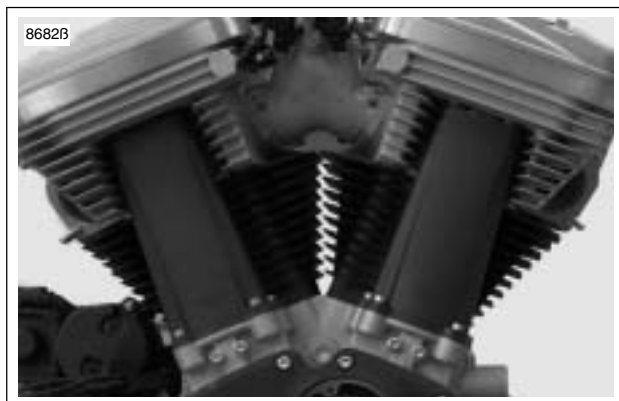
Figure 3-85. Push Rod Locations
