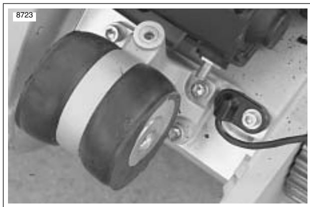
Figure 3-32. Rear Isolator and Mounting Hardware
