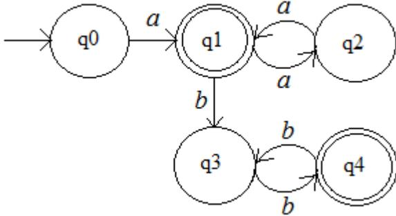
Note that there are other valid solutions. For example, we could redesign the above NFA as follows: replace  $\delta(q1, b) = q3$  with  $\delta(q1, \lambda) = q3$ , make  $q3$  a final state, and make  $q4$  a nonfinal state. The resulting NFA would accept the same language. (However, designing the NFA without  $\lambda$  –transitions makes conversion to a DFA easier...)
