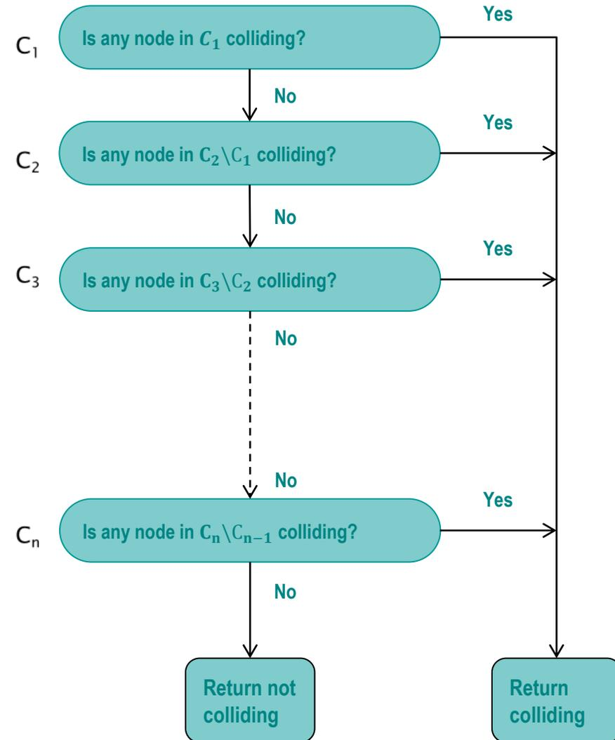
It is important to perform the above checks in a serial manner, otherwise we cannot benefit from the fast collision check algorithm.
