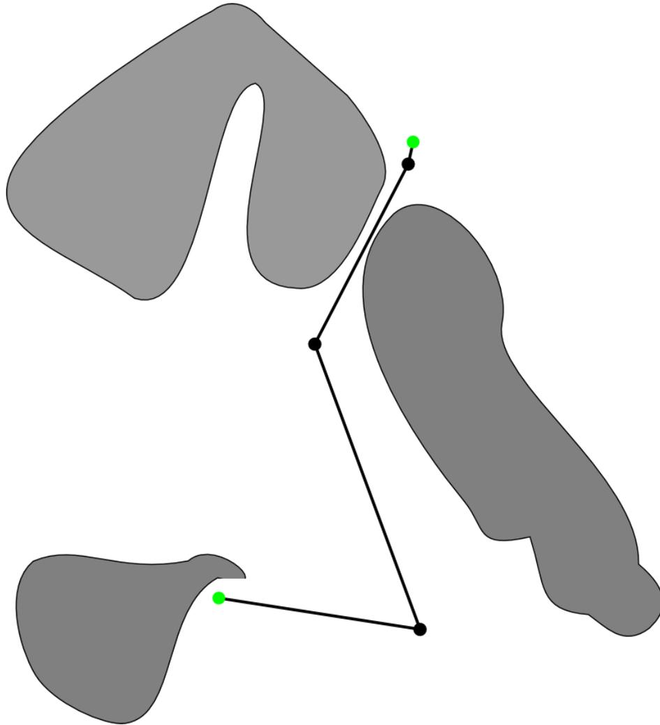
In binpicking applications, final path with collinear purging has usually less nodes than RRT paths that are almost optimized.
