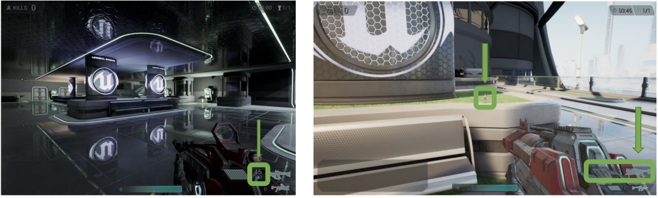
Fig. 1: Visual elements checked automatically after triggering different tests in the official ShootingGame demo from Unreal 4 game engine. For example, in the left figure, the game testing agent used the weapon to fire a fixed number of rounds. The test checks if the visual text representing the new ammo amount is correct. In the right picture, the game testing agent triggered a weapon change test and checks visually if the weapon-cross icon on the screen is the correct one for the new weapon selected and the camera’s zoom level. The new weapon selection should correspond to the icon in the bottom right of the screen.
