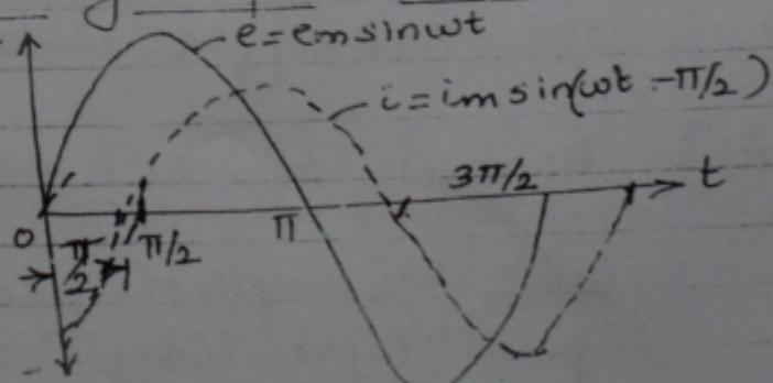
Whenever an alternating voltage is applied to a purely inductive coil, a back emf is produced due to self inductance. This back emf always opposes this change in current in the coil.
