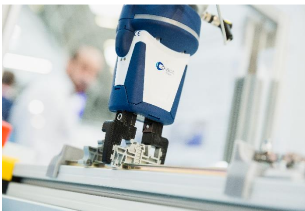
Figure 1 – Mounting process of end clamps in a human-robot collaboration scenario.
