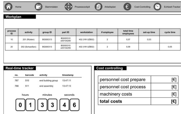
Figure 2 - Basic GUI of the assembly recorder
