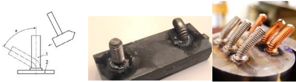
Figure 9 - 60° bending test according to DIN EN ISO 14555 [14].
