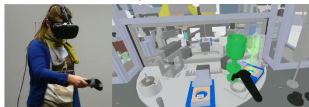
Figure 5 - The Implemented VR-based Mock-Up.
