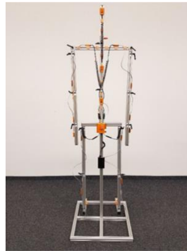
Figure 3 - Human Body Angle Assessment Model (posterior view)
