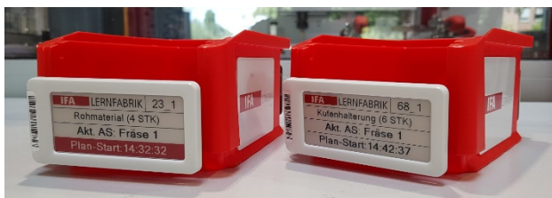
Figure 4 - Loading boxes with two ESL each
