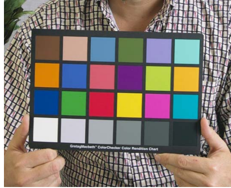
Figure 5: Gretag–Macbeth ColorChecker color chart being held in a portrait setting. (en.wikipedia.org, image by Richard F. Lyon)
