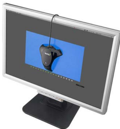
Figure 3: A Datacolor Spyder 3 in position on a monitor (from a Datacolor website).
