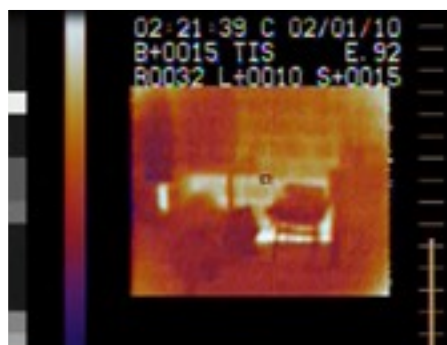
HEAT ESCAPING INTO GARAGE
