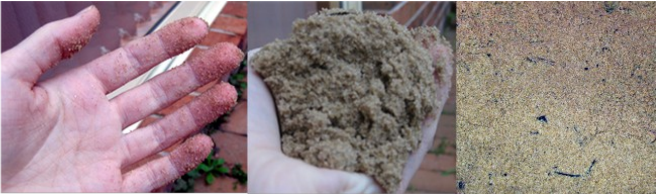
Image: Left to right: grains, pile and lots of (real) sand. The continuum model used in this thesis will not be able to simulate the grains that get stuck to surfaces as shown on the left.
