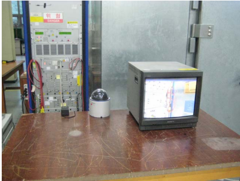
General test set-up for immunity to Surge interference
