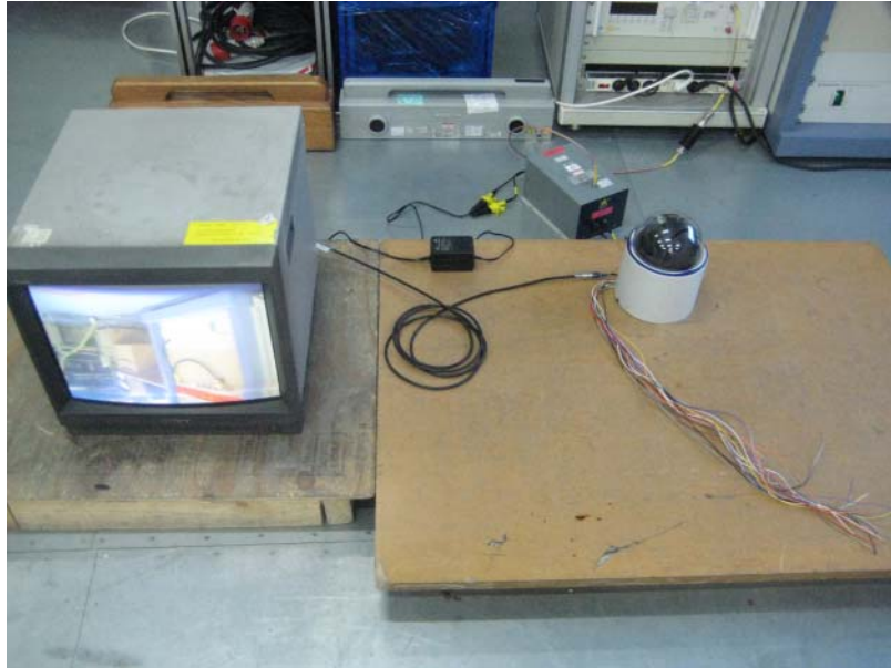
General test set-up for immunity to conducted disturbances
