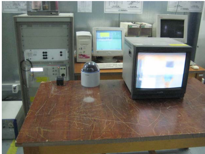
General test set-up for immunity to voltage dips, short interruptions
