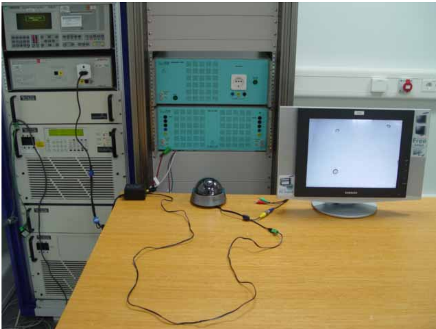
Picture 4. Harmonics & Flicker
